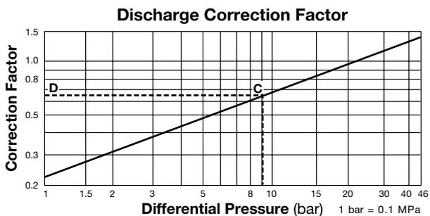
Differential pressure is the difference between the inlet and outlet pressure of the trap.
